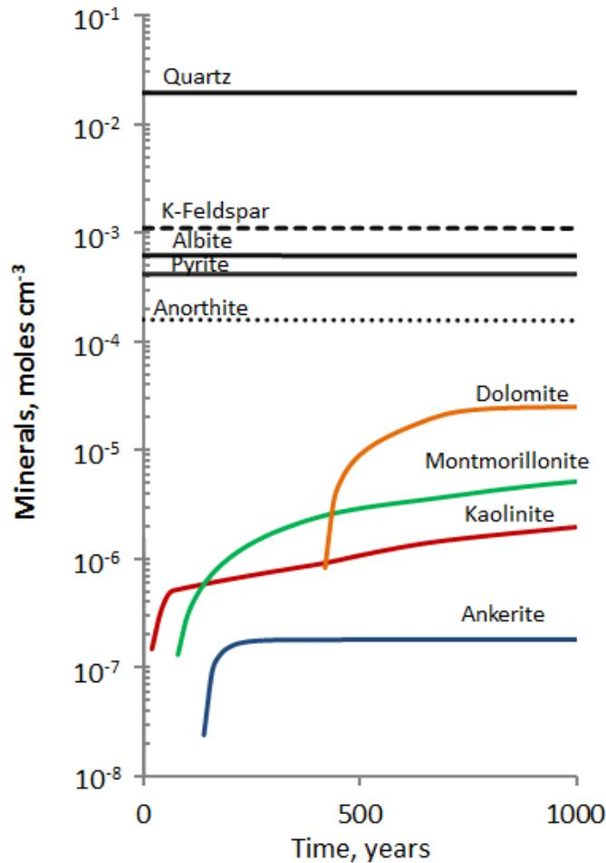
Reactive transport models over 1000 years predict precipitation of minerals kaolinite, montmorillonite, dolomite and ankerite.
